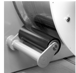
"Seven O'Clock" Roller keeps wire from dragging on plant floor.
