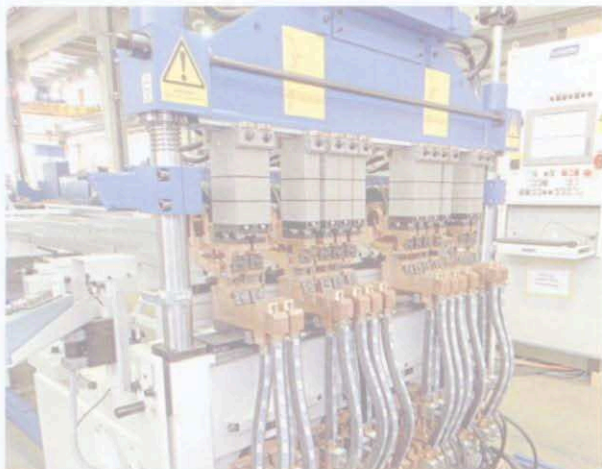
New jig system allows rapid line changeovers on Schlatter mesh welders.
